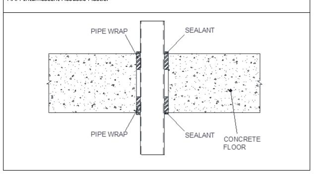
**A.2.1.1 PVC-U** pipes with fischer FiPW-E Pipe Wrap installed within both sides of rigid floor PVC pipes according to EN 1452 with fischer FiPW-E Pipe Wrap.
